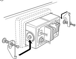
Tighten the end bolts on the clamps (rotate clockwise) so that the clamps press firmly against the inside of the instrument control panel.
